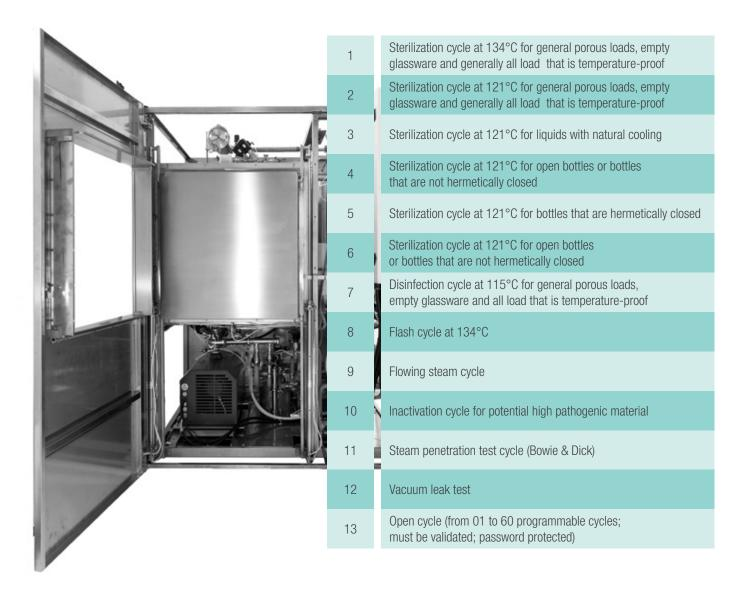
Other cycles can be used for pharmaceutical industry like Crash test cycle And additional cycle can be added and or validated upon requested.
