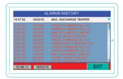
Audio and visual alarms are defined for operator warning; the alarms list includes multilevel alarms with clear message notification; alarm levels are configured based on the level of importance to stop the machine or the cycle as well as just warning notification without affecting the running cycle.
