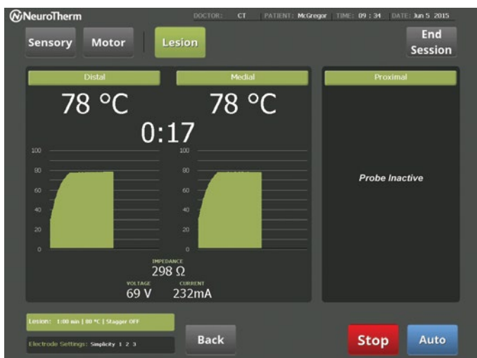
Figure 14. Tap Auto to begin treatment. First, a bipolar lesion is created between the distal and medial electrodes.
