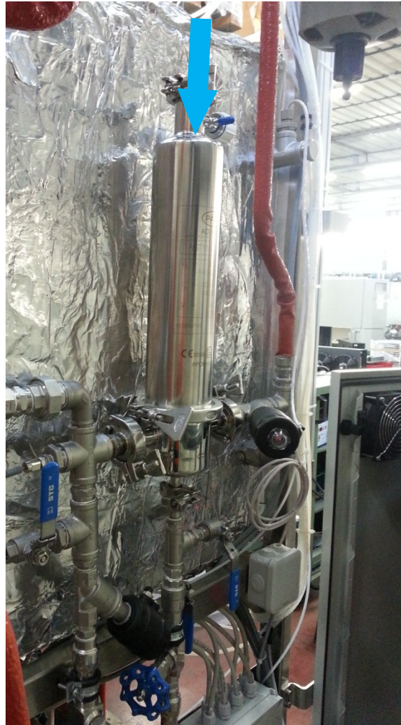
14. Steam generation by direct steam connection to an external source (S).
