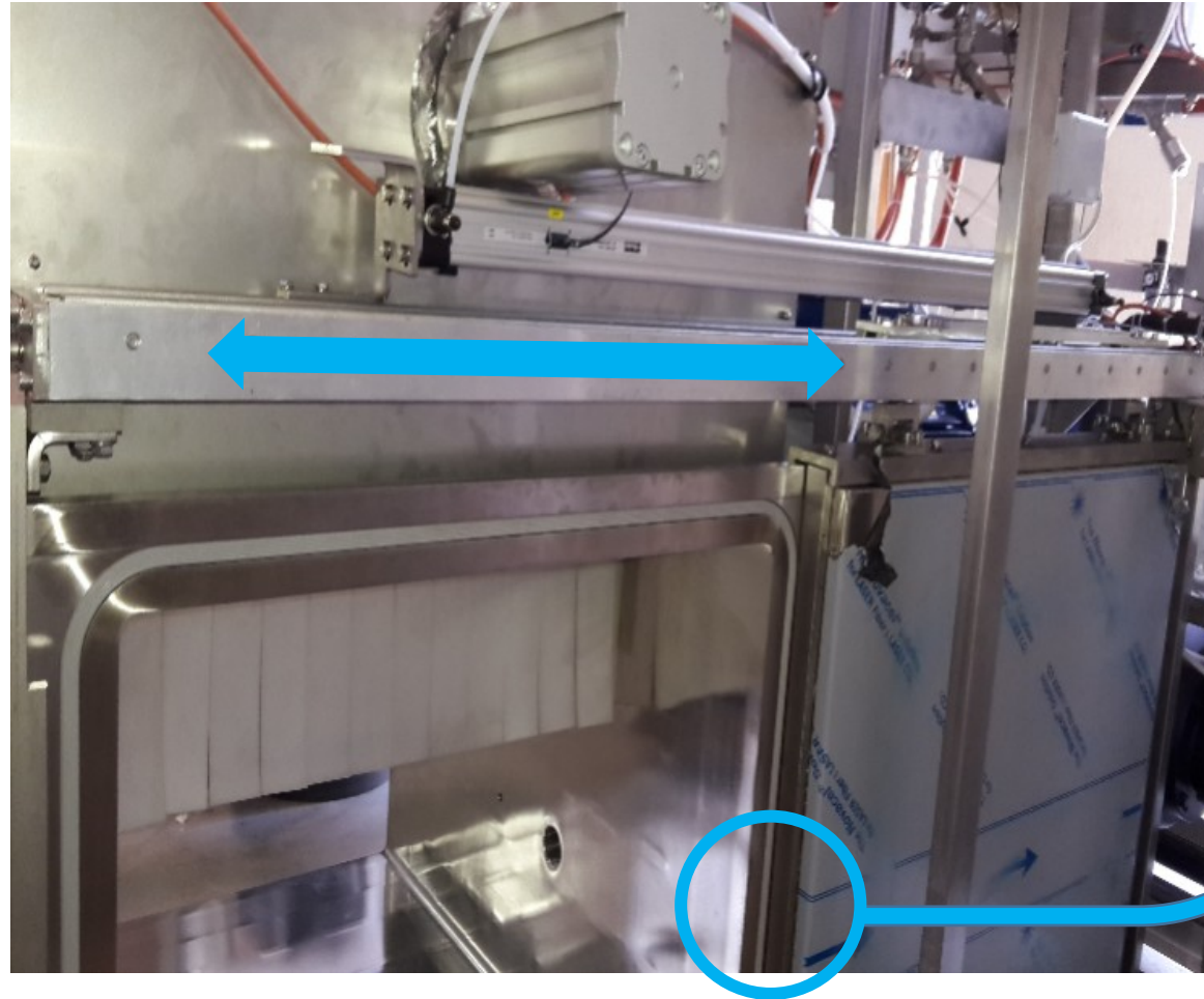
7. Doors horizontal automatic sliding device.
