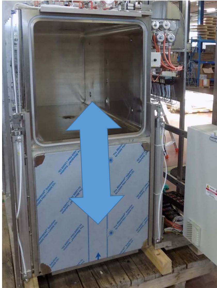
8 Automatic sliding device for vertical door/s.
