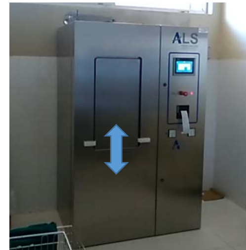
Automatic sliding device for vertical door/s.
