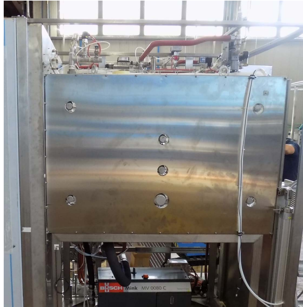
10 Chamber and steam generator isolated with fire retardant mattress, covered with stainless steel panels.
