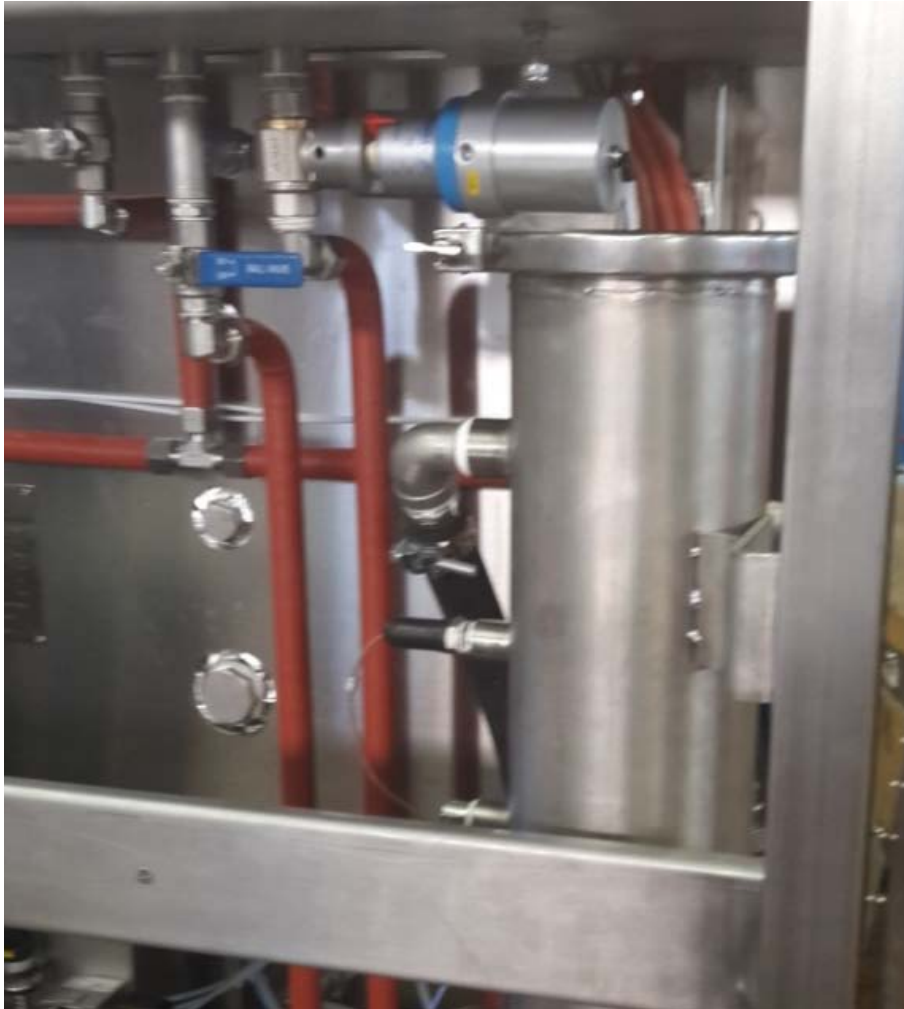
18 Generator water preheating, Energy recovery system and Water generator de-gassing system. (optional)
