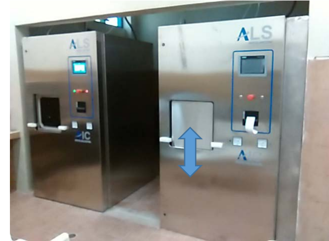
Automatic sliding device for vertical door/s.
