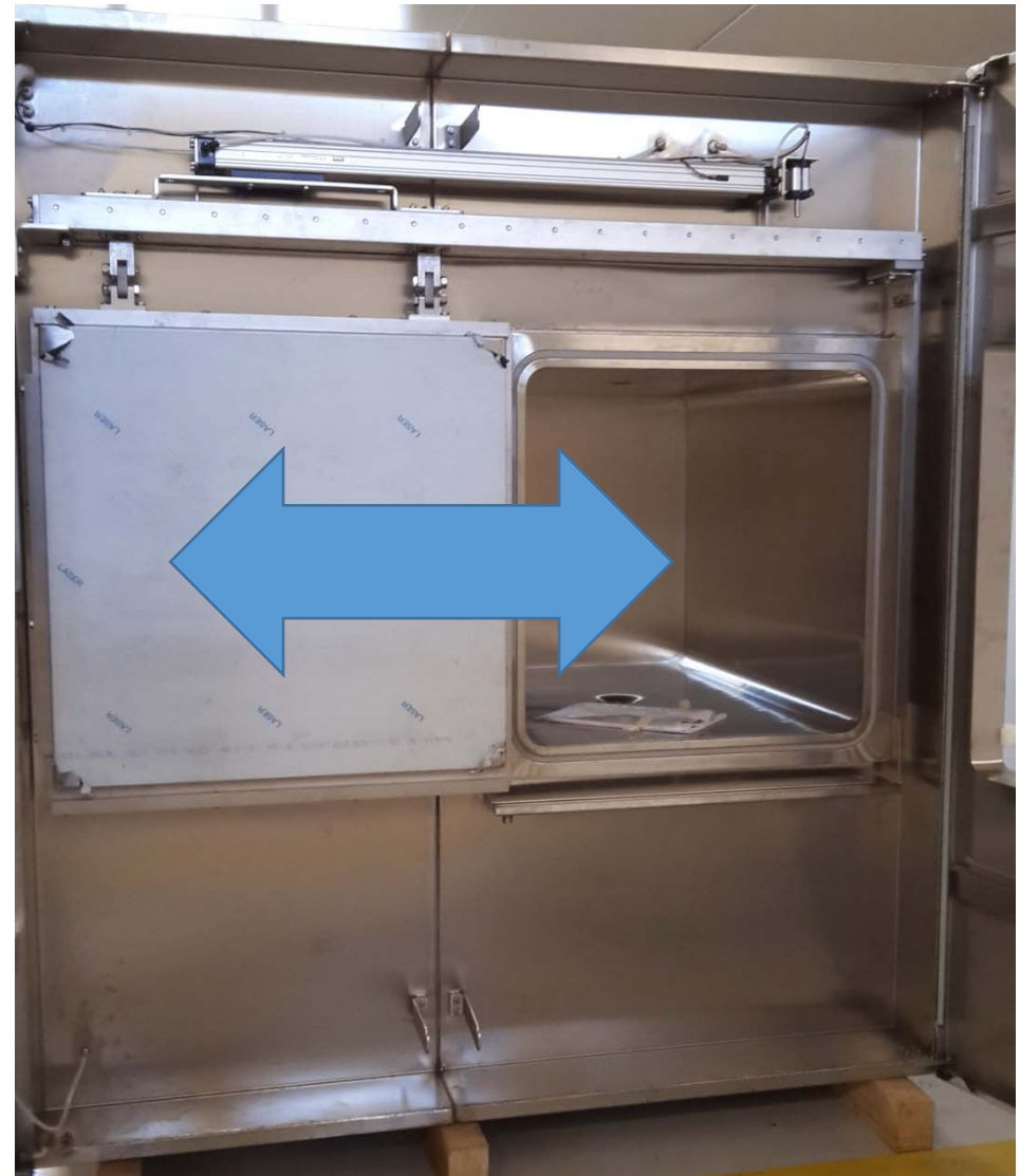
Automatic sliding device for horizontal door/s.
