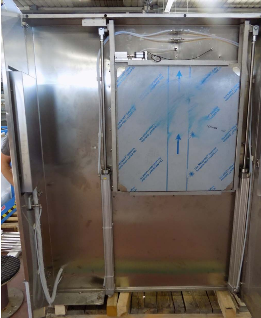
12 Bio-seal shield: separation between sterile side and clean side.
