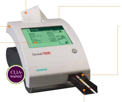
RS-232 serial port allows transmission of results to a personal computer.
