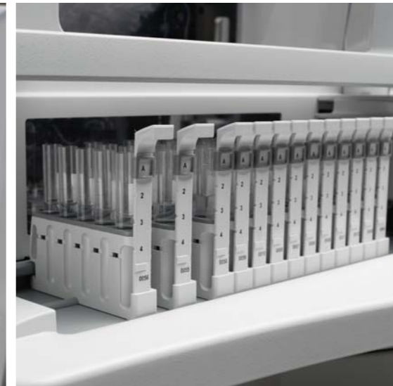
Sample rack holds any size tube
