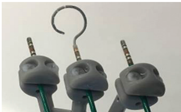
Figure 4: DWL fixture showing the Advisor™ FL circular mapping catheter, Sensor Enabled™ (in center)
